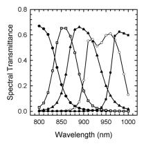
Figure 5. Spectral transmittance of the real interference filters.
